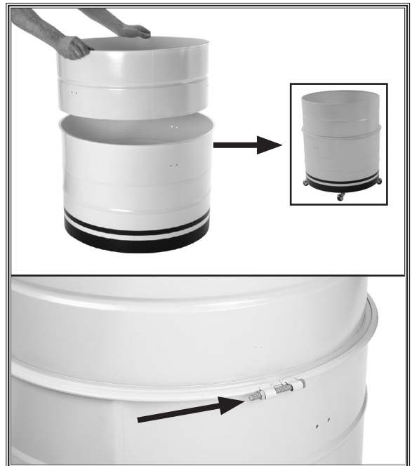
Figure 31. (Top) Connecting upper and lower collection drums, (bottom) drum clamp installed between drums.
